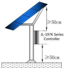
Figure 4. Control Box Location
