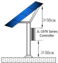
Figure 4. Control Box Location
