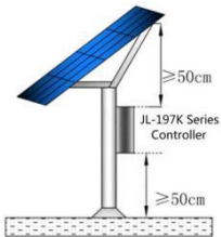
Figure 4. Control Box Location
