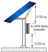
Figure 4. Control Box Location
