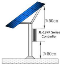
Figure 4. Control Box Location
