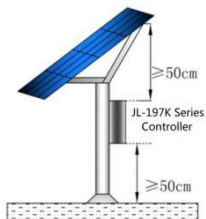
Figure 4. Control Box Location
